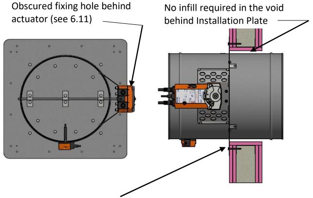
38mm long drywall screws to affix installation plate to metal frame within drywall (see 6.11)
