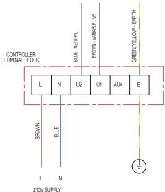
For controllers with TK function add suffix TK. This option is not available with the EL101.
